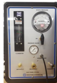
Helmet Test Instrument for 2216 psi air supply
