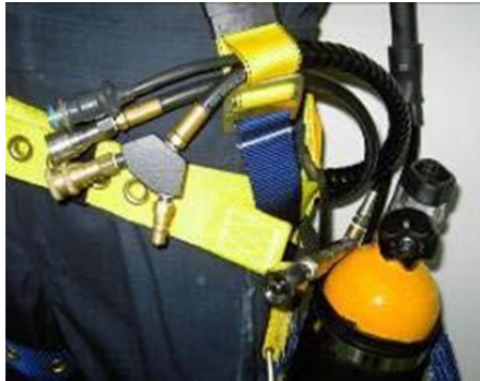
Helmet air hose couplings should be at left side of harness
